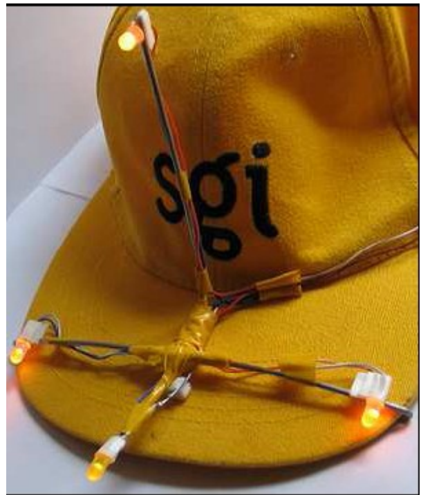
Figure 2, LED's Mounted on a cap
